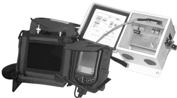
Figure 6. Remote Monitor Kit Connected to a IPS-RDPE-2
